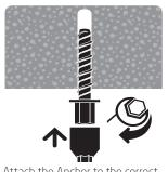
3 Attach the Anchor to the correct size socket driver and install anchor perpendicular to the base material substrate. Be sure not to over torque the anchor. Install with either a socket or cordless impact driver.
